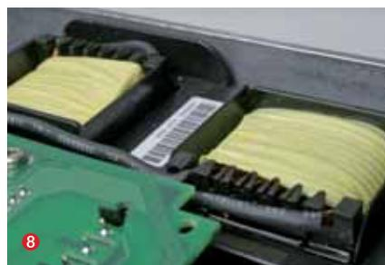
DC coils reduce harmonic noise and protect the drive. Also EMC filters are integrated (meets EN 55011 A2, A1 or B).
