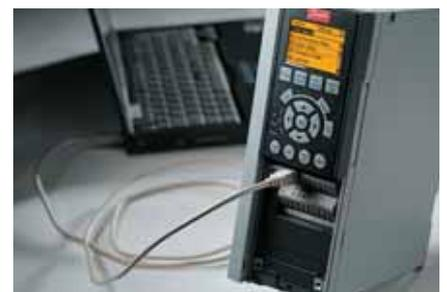
Remote access via fieldbus and USB cable. VLT® Set up Software MCT 10 gives intuitive access to all parameters and has scope features with graphs showing feedback, current, frequency etc. for easy fault finding and documentation.
