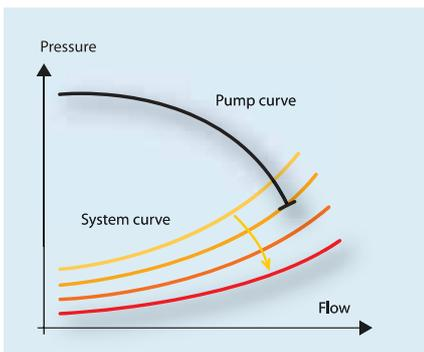
**End of Pump Curve detects breaks and leakage**
