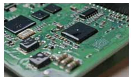
Coated control boards are available for harsh environments.
